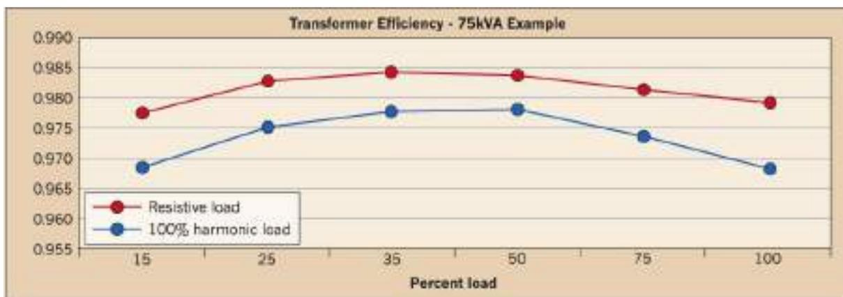
Figure 18 - Change in performance of a transformer on varying harmonic content and load.
