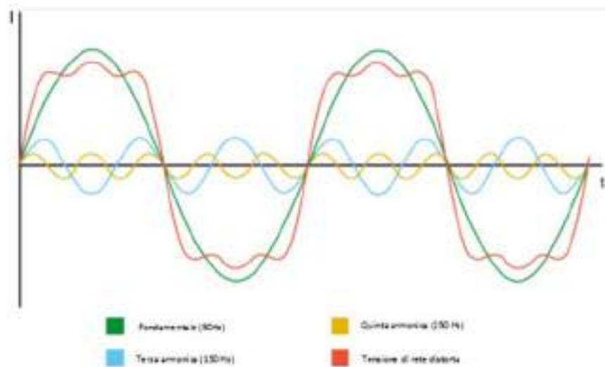
Figure 6 - Distorted current (in red) and its main harmonic components.
