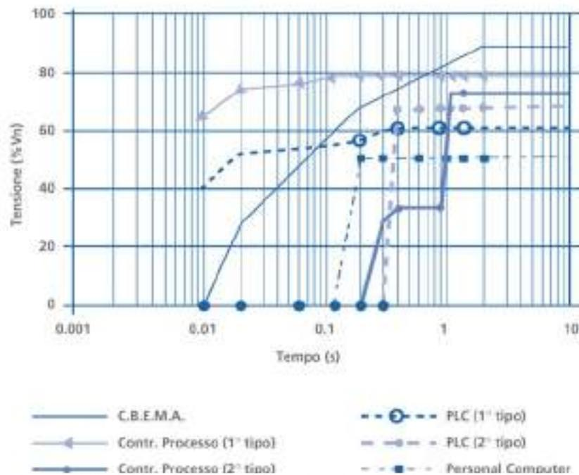
Figure 8 - Susceptibility curves for PCs and control equipment (PLCs and process controllers)
