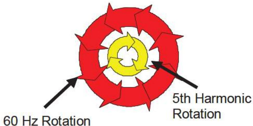
Figure 19 - Breaking effect of the harmonic V in the rotation of a motor
