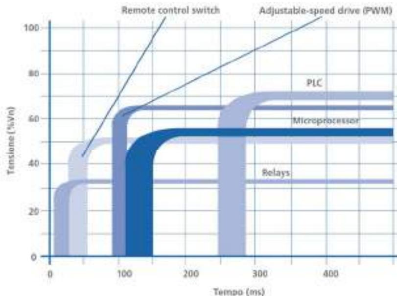
Figure 7 - Susceptibility curves for PLCs, relays, microprocessors and variable speed drives.
