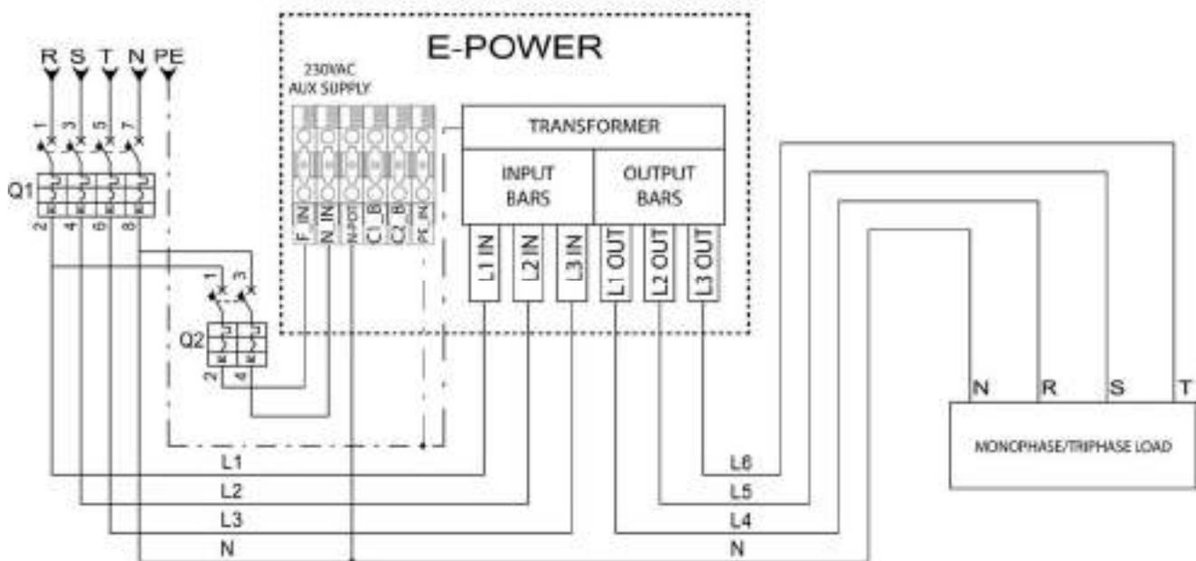
Figure 5 - Typical configuration of a system equipped with E-POWER
