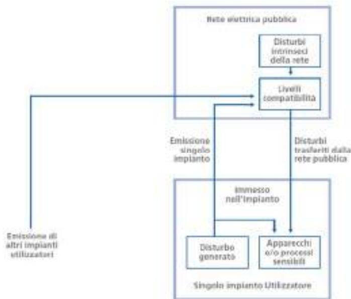
Figure 1 - Layout of the generation and distribution of line disturbances
