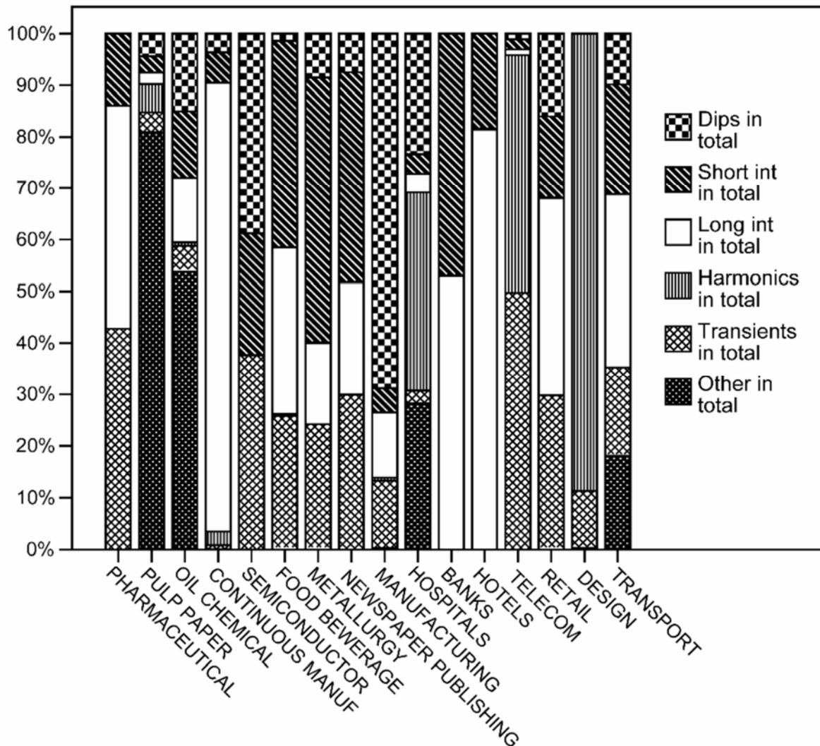
Figure 10 - Breakdown of total costs on the basis of disturbance type.
