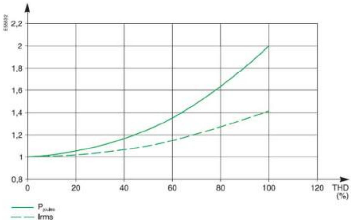
Figure 20 - Increase in the effective value of the current and losses due to the Joule effect in the conductors as a function of THD.
