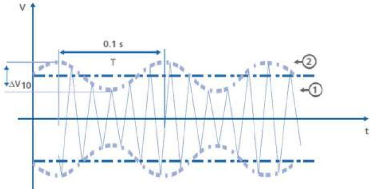
Figure 3 - Example of sinusoidal voltage fluctuation at a frequency of 10 Hz.
