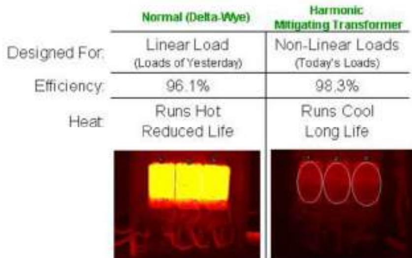
Figure 17 – Thermal effects of harmonics in a power transformer.
