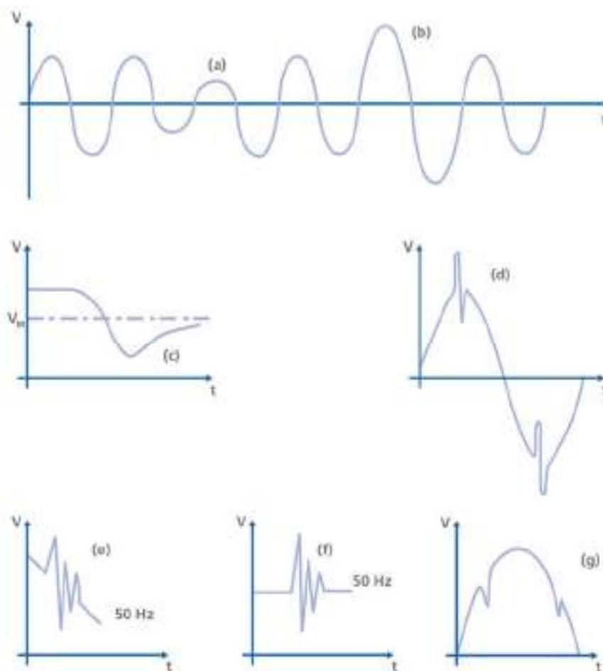
Figure 2 - Diagram of type of variation in voltage amplitude. (a) Voltage dips or flicker; (b) Non-impulsive surge voltages (c) Slow variations (d) Impulsive surge voltages of long duration (e) Impulsive surge voltages of medium duration (f) Impulsive surge voltages of short duration (g).
